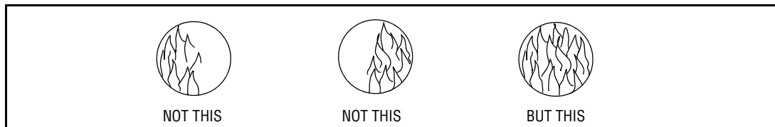
FIGURE 6. FLAME MUST COMPLETELY COVER SIGHT OPENING
