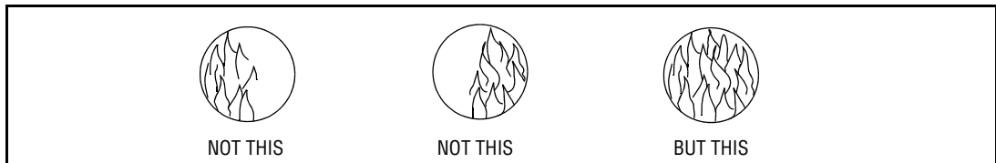
FIGURE 6. FLAME MUST COMPLETELY COVER SIGHT OPENING
