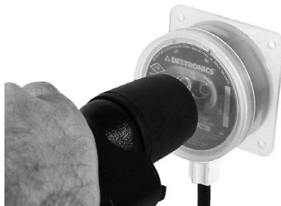
Figure 3—Testing a PM-5MPX with the PSS-MP Test Lamp
