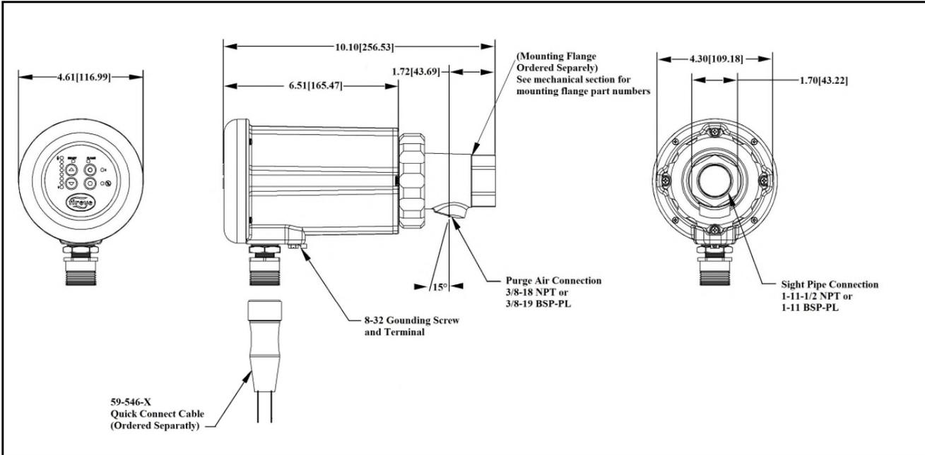
**FIGURE 2. PHOENIX SCANNER in ATEX HAZARDOUS AREA HOUSING (mounting flange kit ordered separately)**
