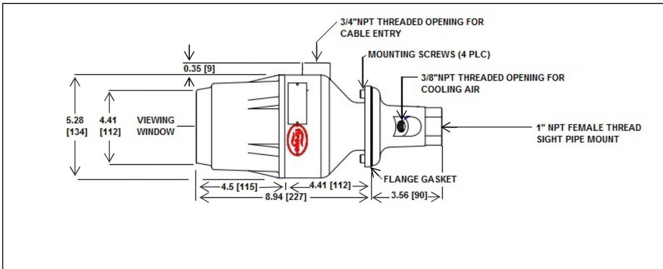
All models of the Phoenix 85UVF1/IRF1-1CEX and 85UVF1-1CEX-K3 flame scanners are housed within an ATEX approved housing for application in Ex II 2 G/D hazardous rated environment. In addition the ATEX housing is designed to meet the requirements of IP66 (NEMA 4X).
