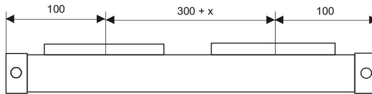
X = stroke can be extended to up to 6 000 mm
