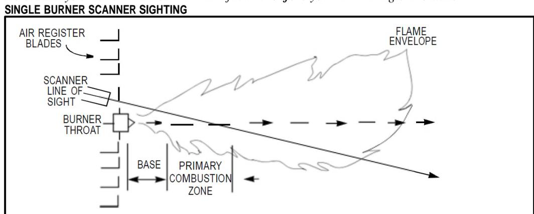
4. Consideration must be given to burner secondary air rotation, some burners have clockwise (CW) air rotation and others have counterclockwise (CCW) air rotation. If combustion air enters the furnace with a rotational movement of sufficient velocity to deflect the ignitor flame in the direction of rotation, position the scanner 10 to 30 degrees downstream of the ignitor as shown in Figure 4 and close to the periphery of the burner throat (See Figure 3).
