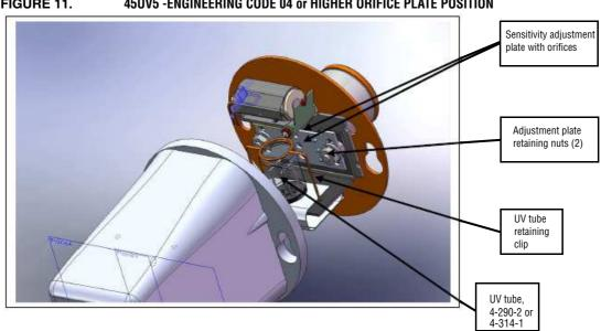
45UV5 -ENGINEERING CODE 04 or HIGHER ORIFICE PLATE POSITION FIGURE 11.
