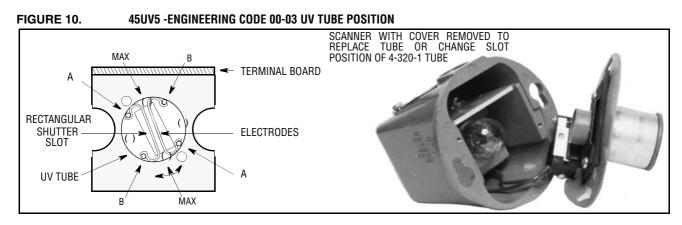
*Note:* To change UV Tube position, pull tube out of eight pin (octal) socket, rotate to desired position, and then insert.
