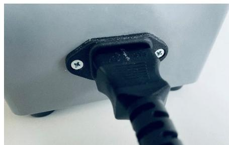
Figure 3- Power connector plugged in
