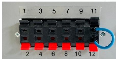
*Figure 4 - Terminal block with jumper inserted to simulate UV radiation with a wavelength of 260 nm.*
