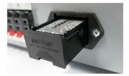
Figure 2 – Battery compartment (opened)
