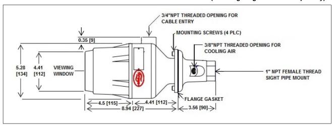
All models of the Phoenix 85UVF1/IRF1-1CEX and 85UVF1-1CEX-K3 flame scanners are housed within an ATEX approved housing for application in Ex II 2 G/D hazardous rated environment. In addition the ATEX housing is designed to meet the requirements of IP66 (NEMA 4X).
