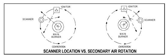
5. If combustion air enters the furnace with a rotational movement of sufficient velocity to deflect pilot flame in direction of rotation, position the scanner 0 to 30 degrees downstream of the pilot burner and close to the periphery of the throat where the ultraviolet radiation is at a maximum. (See Figures 3 and 4).
