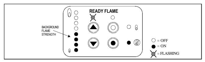
FIGURE 11. Examples of Flame Detection Thresholds (Adjusted for Learned Background Flame)
