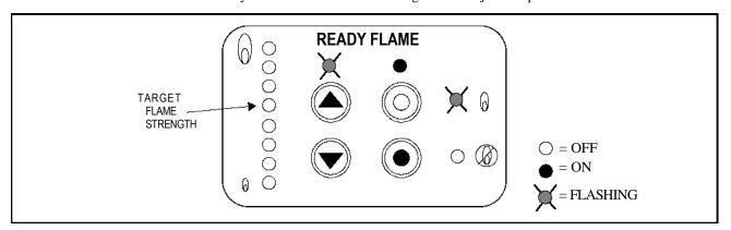
The Flame Strength should BRIEFLY GO BELOW 6 LEDs. If the LEDs stay at 7 or above, add orifices to minimize the signal (see page 29). If the signal strength does not drop below 6 LEDs, then decrease the size of the orifice. This may require some testing to determine the correct size.
