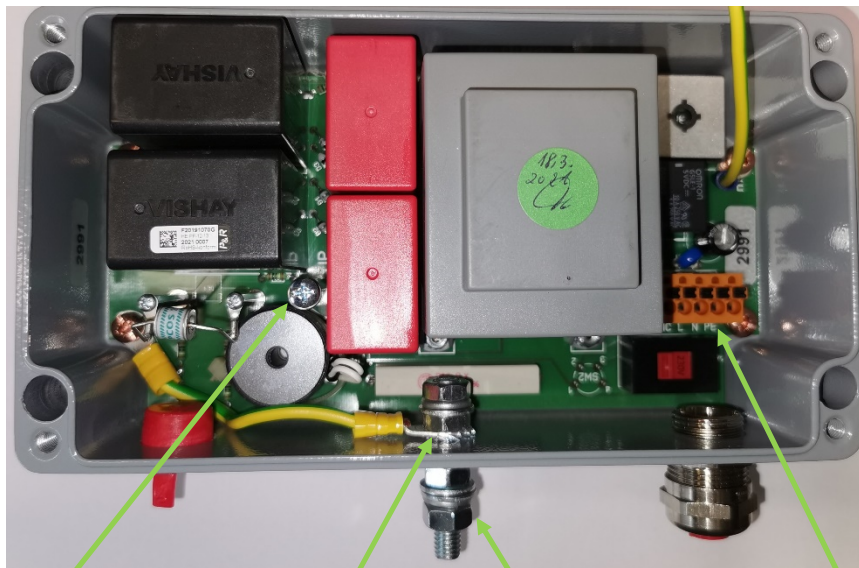
Figure 4: Electrical connection of the high-energy ignition unit ZSH-PP-16
